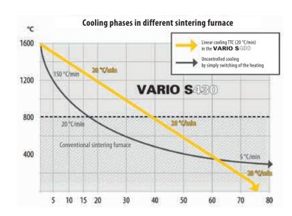
Below this temperature the lift lowers itself by a few millimetres. The thermocouple checks the current temperature in the furnace chamber every second. If the temperature is dropping faster than the programmed cooling rate the electronic controller compensates this deviation by means of targeted reheating or correction of the lift position.
