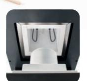
High-quality molybdenum disilicide heating elements reach a maximum end temperature of 1.650°C. Unlike silicon carbide heating systems, heaters of this type are far enough away from their maximum performance limit of approx. 1.800°C. Thanks to this property they attain a significantly longer service life. Each of the four heating elements can be individually replaced in case of damage – an "en bloc" replacement is unnecessary.
